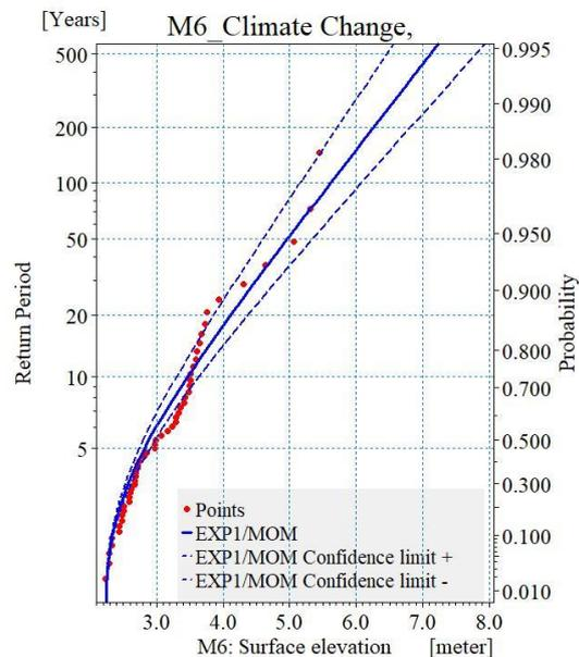
**Figure 10.** Frequency Distribution Curve of Maximum Storm Surge Level of Point M6 (Climate Change Condition)
