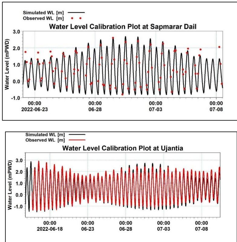
**Figure 4.** Calibration plot of 2D hydrodynamic model
