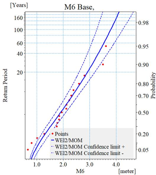
**Figure 11.** .Frequency Distribution Curve of Maximum Significant Wave Height of Point M6 (Base Condition)
