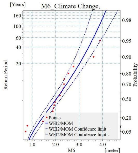
**Figure 12.** .Frequency Distribution Curve of Maximum Significant Wave Height of Point M6 (Climate Change Condition)
