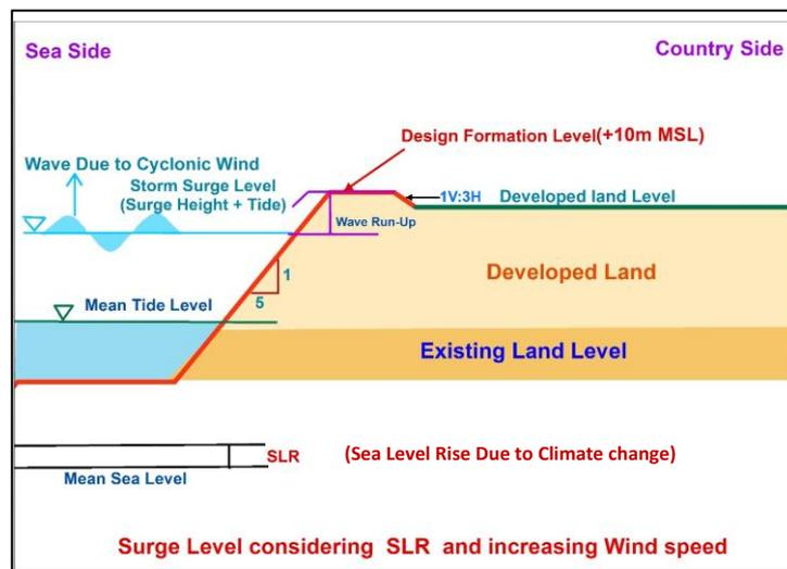
**Figure 16.** A typical computation for fixing embankment crest level (source: IWM)
