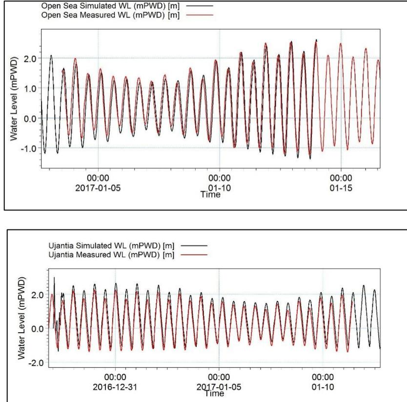
**Figure 5.** Validation plot of 2D hydrodynamic model
