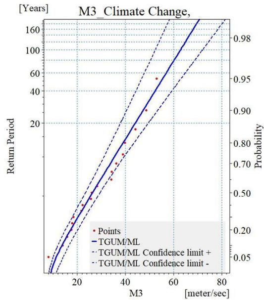
**Figure 14.** Frequency Distribution Curve of Maximum Wind Speed of Point M3 (Climate Change Condition)
