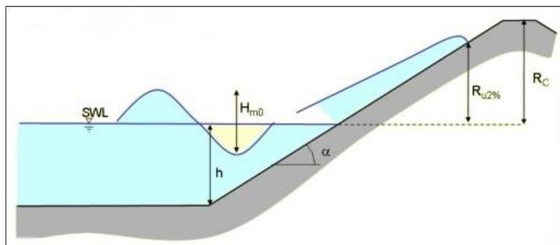
**Figure 15.** Definition of the wave run-up height  $R_{u2\%}$  on a smooth impermeable Slope (Source: Eurotop Manual, 2007)
