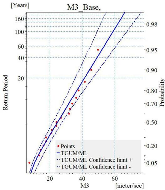
**Figure 13.** Frequency Distribution Curve of Maximum Wind Speed of Point M3 (Base Condition)
