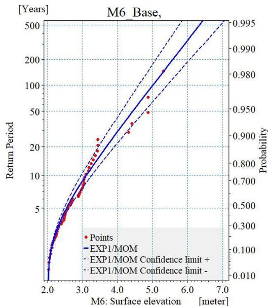
**Figure 9.** Frequency Distribution Curve of Maximum Storm Surge Level of Point M6 (Base Condition)
