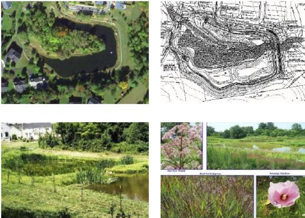
Figure 6. Aerial image and engineered drawing (cross hatch area is preserved forested wetland habitat) of regional horse-shoe pond showing retention areas with pre-treatment cell at pond input and transition habitat
