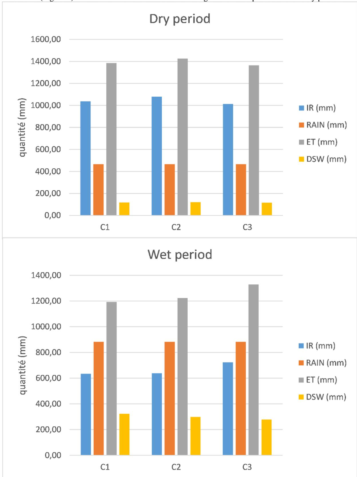
Figure 7. Water balance for the three fields in dry and wet periods
