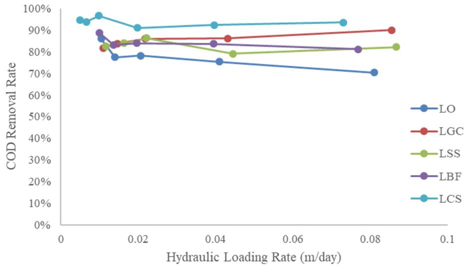
**Figure 2.** COD removal rate from wastewater for the five lab-scale CWs
