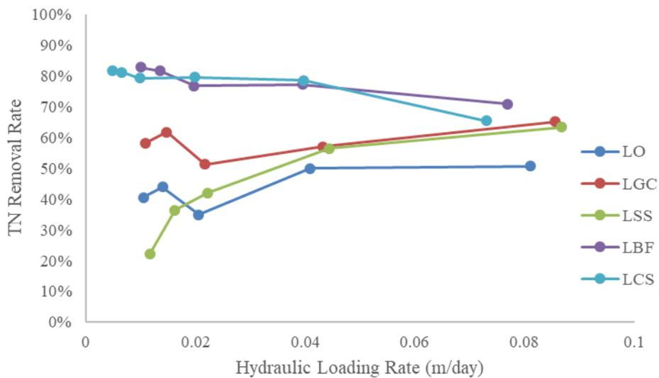
**Figure 4.** TN removal rate from wastewater for the five lab-scale CWs
