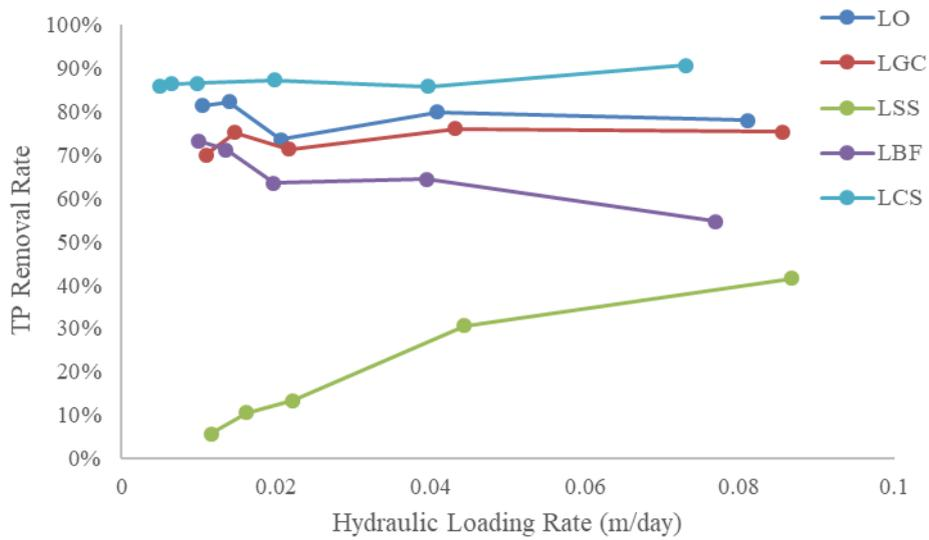
**Figure 3.** TP removal rate from wastewater for the five lab-scale CWs
