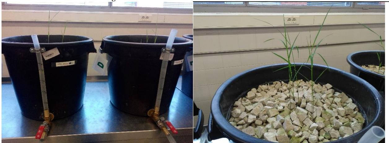
**Figure 1** – Photographs of the experimental lab-scale constructed wetlands setup
