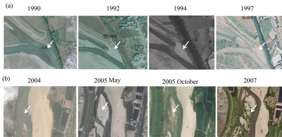
**Figure 4.** Contiguous observations made from aerial photographs at sediment deposited location in the Sagami River (a) and Kizu River (b) (the arrows indicate the sediment deposited location)
