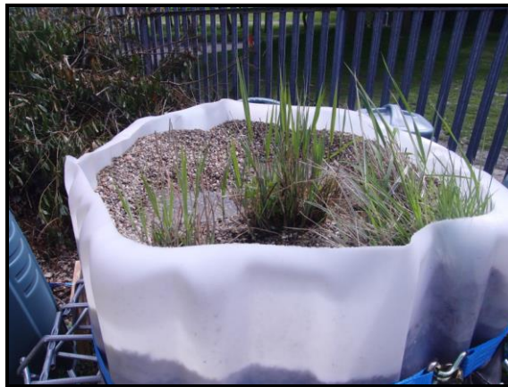
Fig. 2. An overhead photo of the prototype wetland at the Nottingham Trent University. The basis of the module was an IBC container.
