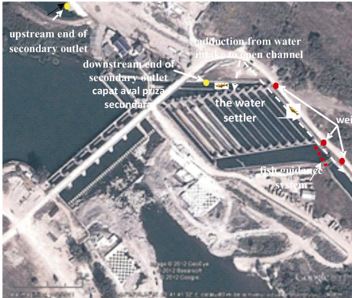
Figure 13. Scheme presenting the location of the fish migration system between gates (Image source: [6])
